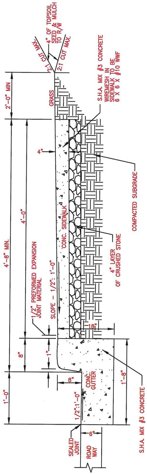
COMBINATION CURB, GUTTER AND SIDEWALK
