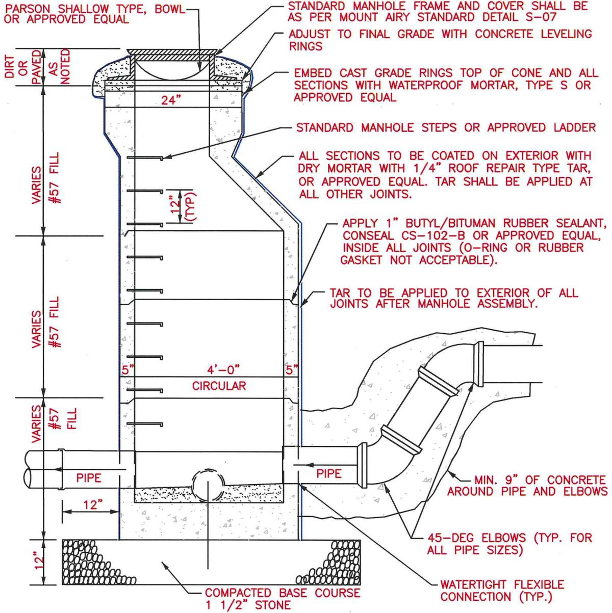
**PRECAST CONCRETE DROP MANHOLE WITH "C" CONNECTION**
