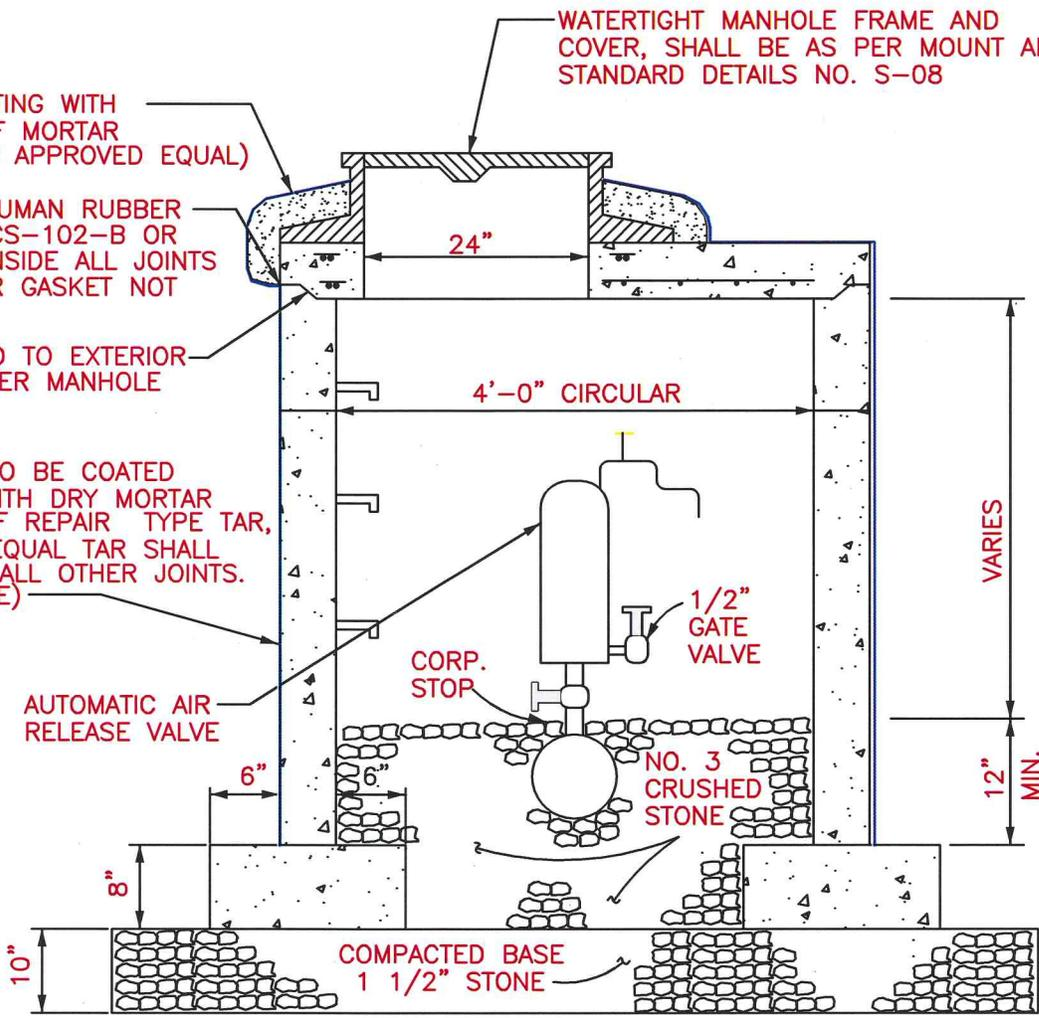
EMBED CASTING WITH WATERPROOF MORTAR (TYPE S OR APPROVED EQUAL)
