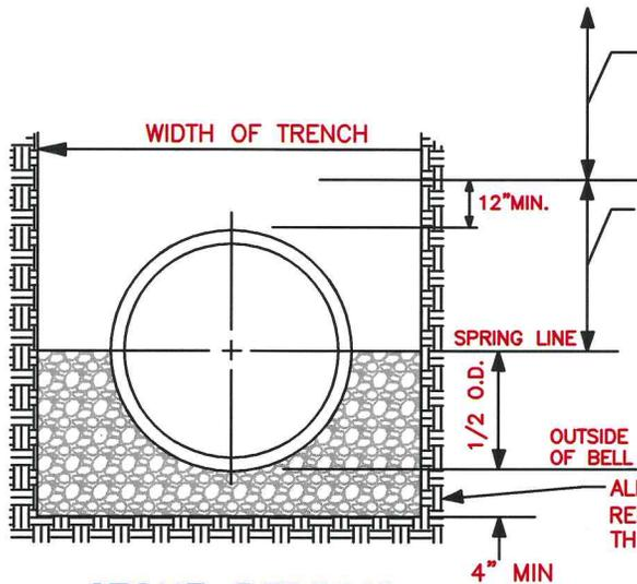
PLACE BACKFILL AND COMPACT TO DENSITY REQUIRED WITH MECHANICAL TAMPER.
