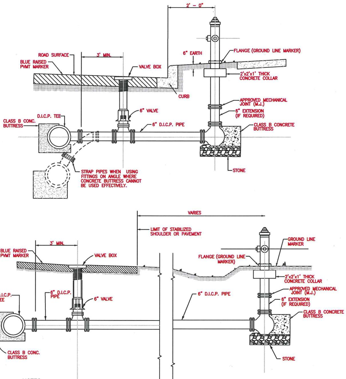
STRAP PIPES WHEN USING FITTINGS ON ANGLE WHERE CONCRETE BUTTRESS CANNOT BE USED EFFECTIVELY.
