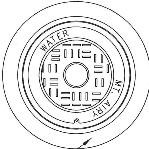
THE FRAME AND COVERS SHALL ALL BE MIN. 420 TRAFFIC TYPE, AND THE COVER SHALL HAVE THE WORDING AS SHOWN. PICK HOLES SHALL BE WATERTIGHT.
